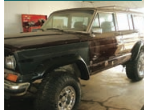
12 As you can see here, the rear flares do not fit nearly as closely as the front ones did. This had me worried at first, but in the end it turned out ok. Just have to go slow and contive to trim the flares until they fit nicely.
