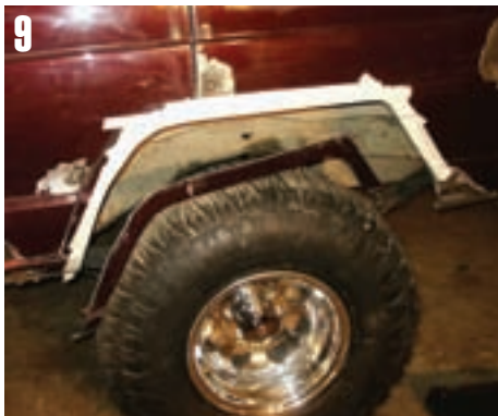
9 This picture shows that I cut at the first body line above the wheel arch. I cut this equal amount all around the wheel opening.
