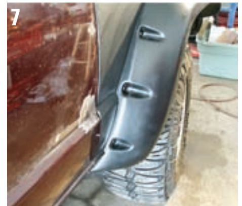
I just continually fit and trimmed the flares until I was happy with the contour. I must have had these flares on and off the truck 10-15 times each with trimming each time.
