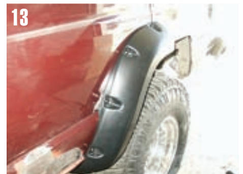
13 For the flare on the door, I just lined it up with the other half, and trimmed along the body and rockerpanel on the front edge. I also cut a chunk out of the underside of the flare so that it does not bow out when closing the door. And that is it. Just repeat for the other side.
