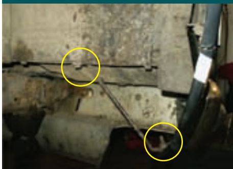
There are two brackets on the back side of the fenders that will need to be removed/undone.
