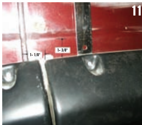
11 Here is what I have come up with for measurements to install the flare on the quarter panel.
