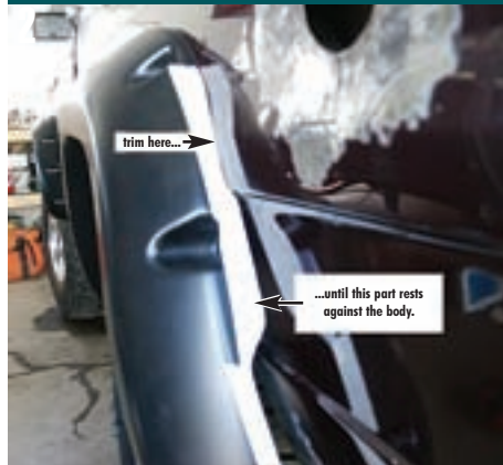
12 As you can see here, the rear flares do not fit nearly as closely as the front ones did. This had me worried at first, but in the end it turned out ok. Just have to go slow and contive to trim the flares until they fit nicely.
