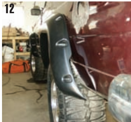
12 As you can see here, the rear flares do not fit nearly as closely as the front ones did. This had me worried at first, but in the end it turned out ok. Just have to go slow and contive to trim the flares until they fit nicely.
