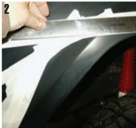
I started with the front flares by holding them up against the fender and getting a rough idea on what needed to be cut out. I took the time to lay tape down as a guide for my cuts. The tape both marks the lines to be cut and protects the paint from getting marked up.
