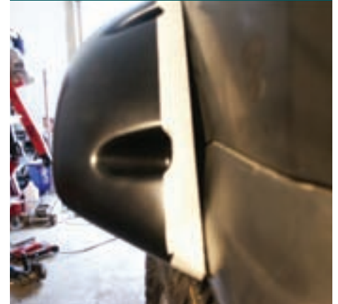
I just continually fit and trimmed the flares until I was happy with the contour. I must have had these flares on and off the truck 10-15 times each with trimming each time.
