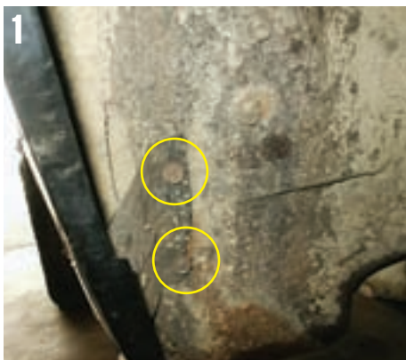
There are two brackets on the back side of the fenders that will need to be removed/undone.
