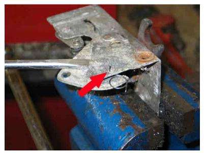
Once the existing spring has been removed, using a pair of needle nose pliers you will fish one end of the spring into the hole shown here on the left.
