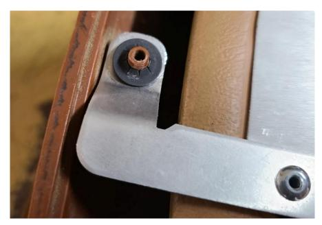
Install the door pull to the door via the #14 screws that were taped to the inside of the door pull with a philips screwdriver. Angle the screwdriver with the handle end lower to hit the screw.
