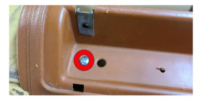
Use the included rubber washers to retain the #14 screws in the aluminum brackets with the threads facing the door panel.
