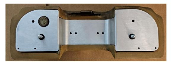
Using the provided 1/8" rivets, rivet the trim brackets to the aluminum support. Install the plastic screws and snug the aluminum to the door pull. Be careful not to overtighten theses screws, the longer screws ('B') go in the outer holes and shorter screws ('C') go in the inner holes. Snug the trim brackets to the trim via the machine screws ('G').
