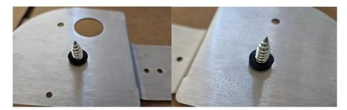
Install the support by pushing the middle in first, then the support will pop snugly into the center section of the door pull between the vinyl sides. Use the supplied 3/4" #8 screws for the outer holes. Use the 5/8" #8 screws in the outer 2 inner holes (the 2 inner-most holes were used in the factory press for alignment and can be ignored).
