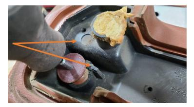
Use the supplied rubber washers to retain the #14 screws (see 'D' below) in the aluminum brackets with the threads facing the door panl.
