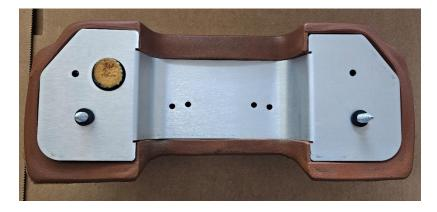
Install the support into the door pull and fasten with #8 screws. The shorter 5/8" length screws (see 'C' below) are used in the outer middle holes and the longer 3/4" screws (see 'B' below) are used in the outermost holes.
