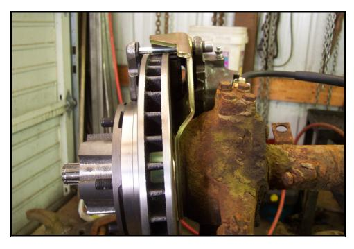
Reinstall locking hub. At this point, the snap ring will no longer fit, as this kit moves the wheel hub outward in relation to the axle shaft.
