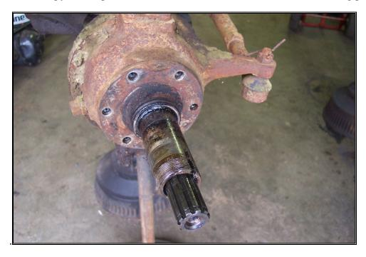
This is as far as you NEED to tear down, but while you are here, it is also a good time to replace leaky wiper seals and U joints.
