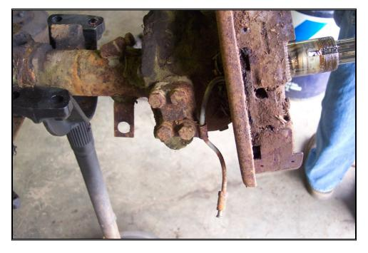
Remove the 6 qty 9/16" spindle bolts, disconnect brake line and remove backing plate.
