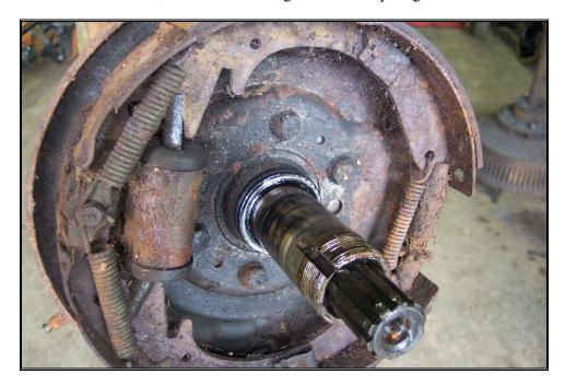
Remove spindle nut, locking washer and inner spindle nut. At this point, you should be able to pull the hub from the spindle.
