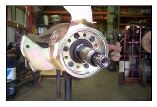
Install caliper bracket using only two bolts (pointed about 45\* toward the rear of the vehicle) and install caliper to check for knuckle clearance. Also make sure bleeder is positioned at the highest point possible, as this will allow trapped air to escape as you bleed your brakes. Some of you will have the caliper contact the knuckle; if the caliper touches the knuckle, you will need to grind the knuckle to allow the caliper to adjust inward as the pads wear.
